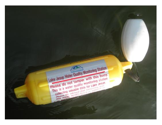
Figure 2-3. Floating Buoy Used to Identify Seepage Monitoring Sites.
