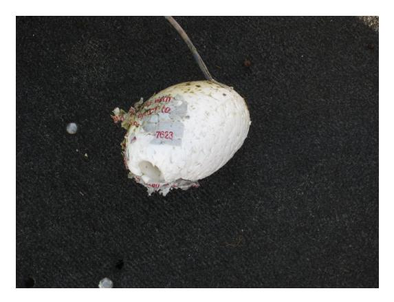
Figure 2-4. Example of Bite Marks on Seepage Meter Floats.
