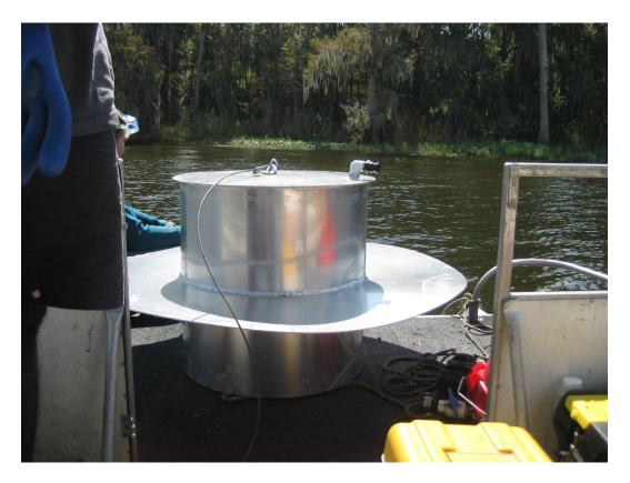
Figure 2-2. Typical Seepage Meter Used in Lake Jesup.
